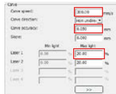
**Note:** The power is inversely proportional to engraved result, which means that with the same power, the faster the speed is, the shallower the engraved depth is.
