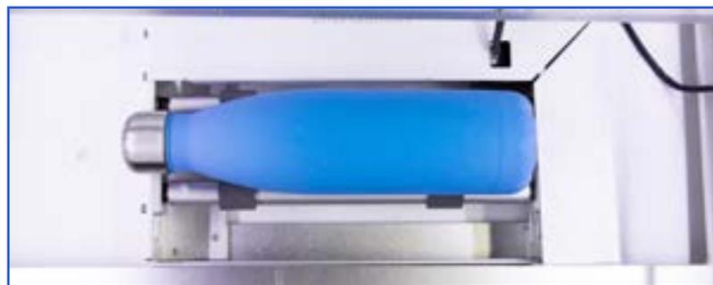
2 Put the bottle onto the roller;
