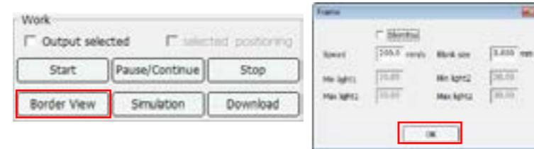
**Note:** If you check "Idemitsu" option, the laser nozzle will draw the moving range using the set power parameters.
