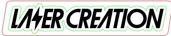
1 Determine the result you want. As the pattern shown above, we want red path to be cut out, green path to be engraved in line (Low-power half cut without cutting through), and black path to be engraved;
