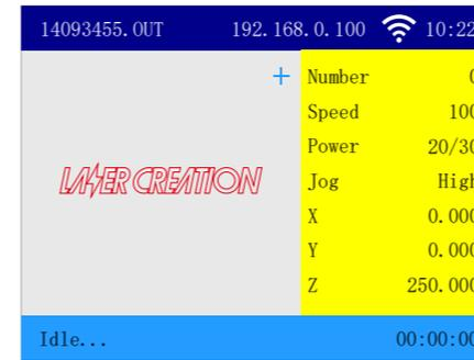
6 When the image has been sent to the machine, you will hear a beep and see the image is on the control panel;
