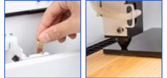
8 Use the acrylic board to adjust the height of laser nozzle. It is the right height when the laser nozzle just touches the board;
